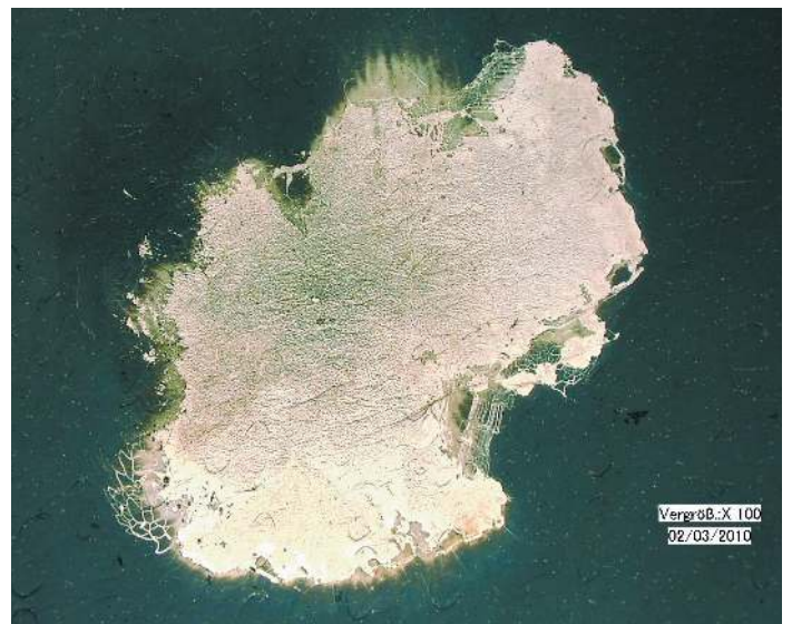
Self-healing event in typical metallized film
