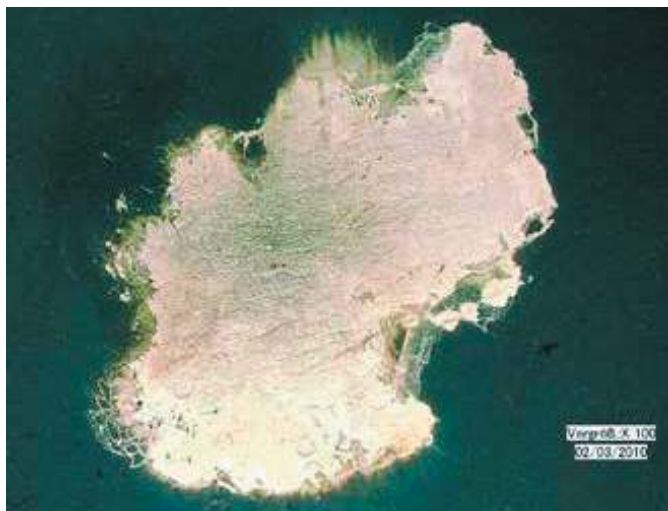
Self-healing event in typical metallized film
